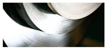
COLD-ROLLED STAINLESS STEEL NARROW WIDTH
