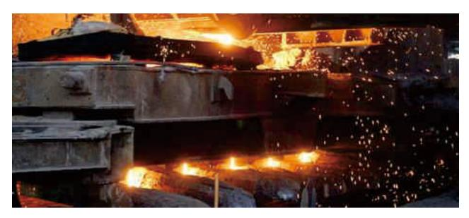
meets standards, raw elements such as sulfur, phosphorus and carbon elements are removed, while alloying elements are added to obtain the correct chemical composition according to the standard.
